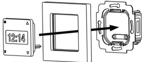
Connect the power unit to the mains and secure it in the flush-mounted socket. Attach the the display, including the frame. Thanks to its total dimensions of 50 x 50 mm, the Selvetimer Plus will fit into a wide variety of switching devices made by leading manufacturers. A suitable adapter will mostly be required.
