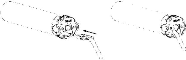
For uninstalling the pluggable cable, de-energise the pluggable cable first. Open the plug lock through the lateral opening at the motor head. This can be done with a screwdriver or a special release tool. Press on the locking clip from both sides and carefully pull out the pluggable cable until the plug comes loose and the pluggable cable can be removed.
