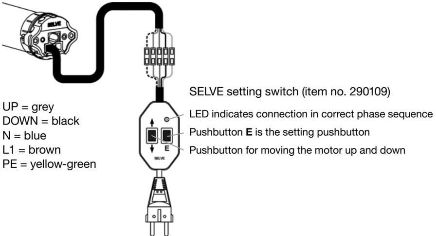
**Caution:** Always connect L1 (= brown) to the permanent voltage supply 230 V even if the motor is only connected for adjustment purposes with a switch or a setting switch.
