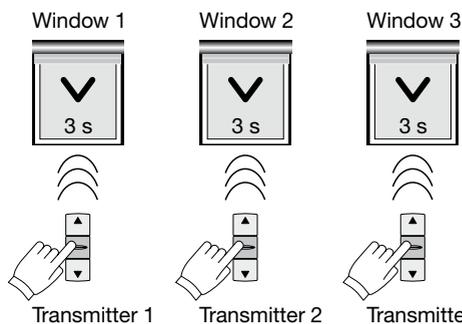
Every motor moves randomly only for 3 seconds within about 2 minutes. The motor in question must be stopped by the selected transmitter during the movement.
