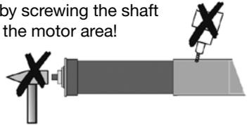
4. Attach the shaft with the motor and the shaft cap in the bearings. Do not bend the motor cable and aerial and place them so that neither the aerial nor the motor cable cannot be damaged. Do not place the aerial parallel to the motor cable. The aerial must not be shortened or extended. To keep water from getting into the motor, place the motor line in a bend direction downwards, so that any water can drip off.
