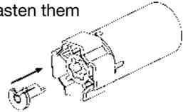
2. Push the motor into the shaft in a positive-locking way. The motor must not be subject to any impacts. Crown and coupling adapters must not have any play inside the shaft.
