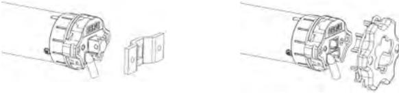
Furthermore, different flanges or mounting plates can be pre-screwed. In case of square support, there must be a mechanical stop behind the motor bearing, in order to avoid axial movement of the square.
