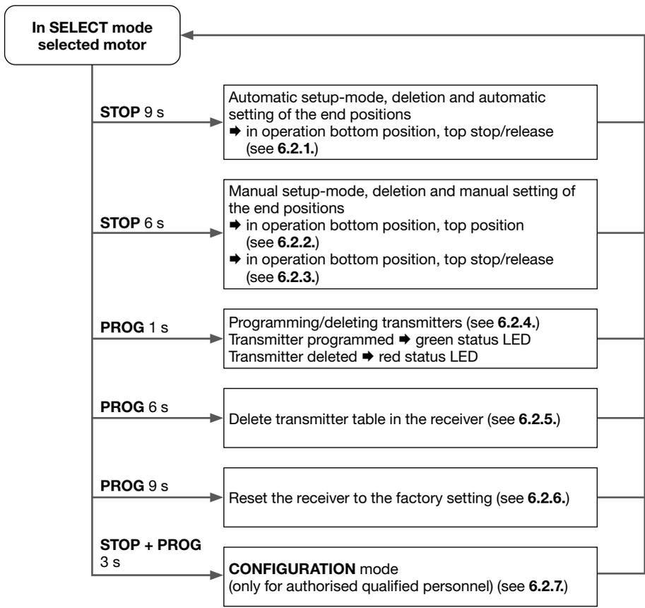
**Note for settings under point 6.2.:** The motor must be selected for this setting with a transmitter in **SELECT** mode (Status LED flashes slowly in orange). After completing the setting, the motor is still selected (see point 6.).
