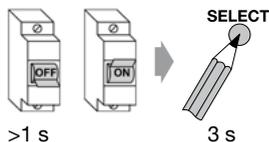
1. Interrupt the voltage supply of the receivers for > 1 second. The receivers can be found within the next 4 minutes.
