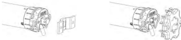
Furthermore, different flanges or mounting plates can be pre-screwed. In case of square support, there must be a mechanical stop behind the motor bearing, in order to avoid axial movement of the square.
